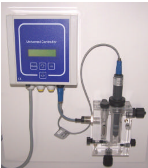
ME5090 Controller connected up to the PEF1 Flow Through Cell
